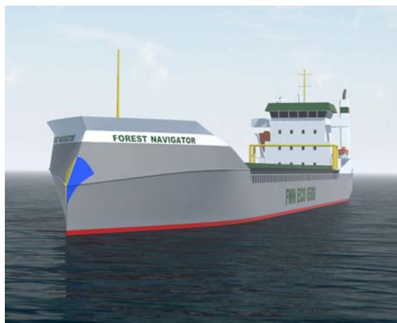
New ECO6500 ship design from ForestWave with Ecospec CSNO x emission control system
